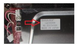
Fanuc i-series CNC controls such as 16i, 18i, 21i, and 0i utilize LCD displays. These LCD display units are NOT made by Fanuc rather are supplied by such LCD makers as SHARP®. Therefore, if you need a replacement LCD, you need to identify the manufacturer's part number on the LCD itself.
