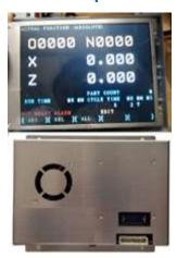
Is the CRT monitor on your Fanuc control taking a while to "warm up" at power on? Or is it becoming too hard to read? Why not replace it with LCD replacement from KFAS? The unit is designed as a "drop-in replacement" and no modification required. We have a limited quantity of LCD replacement for Fanuc A61L-0001-0093 CRT units (commonly used in Fanuc 0, 16, 18 and 21 controls).
