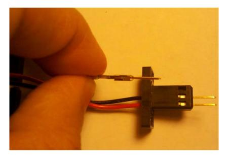
3) Insert the new wires into the connector. Pay attention to the location of each wire as shown below. Inserting the wires in wrong location can cause damage to the fan and/or the Fanuc drive unit!!
