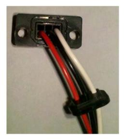
2) To remove the pins from the connector, pull out the corresponding wire while pushing down on the pin as shown below.
